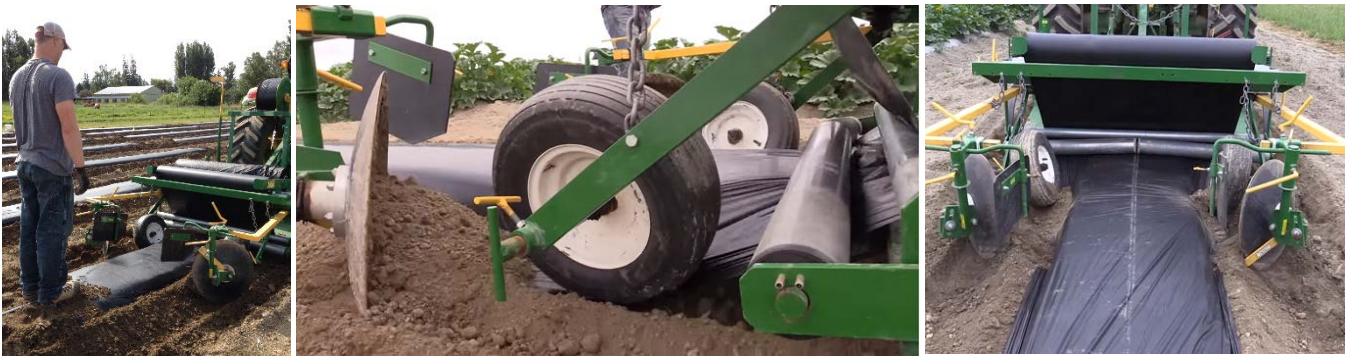
Figure 3. Step on the mulch before the tractor starts moving forward to hold the mulch in place (left); mulch layer roller bars should move freely and wheels should barely touch the mulch (middle); the mulch should be loose on the bed to avoid ripping (right).
