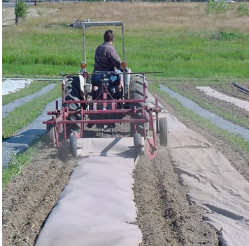
Figure 1. Laying paper mulch with conventional mulch laying equipment; drip tape was laid at the same time in 2 rows under the mulch.
